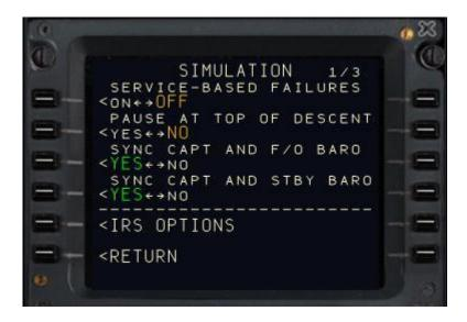
• We recommend that the F/O's altimeter and Standby altimeter syncs to the Captain's altimeter as shown below.
